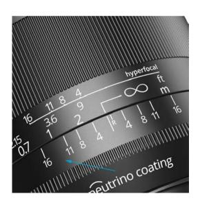
The depth of field scale provides a visual reference for the range of maximum sharpness in your photos at a given aperture and focus setting. It allows you to determine the plane of focus, within which objects in your image will be at their sharpest.
