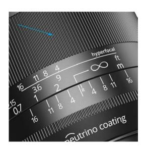
The focusing ring moves the internal focusing elements of the lens to achieve the desired focal point. You can focus visually while looking at your subject in the viewfinder or LCD screen or by using the distance, depth of field or hyperfocal scales on the lens barrel.
